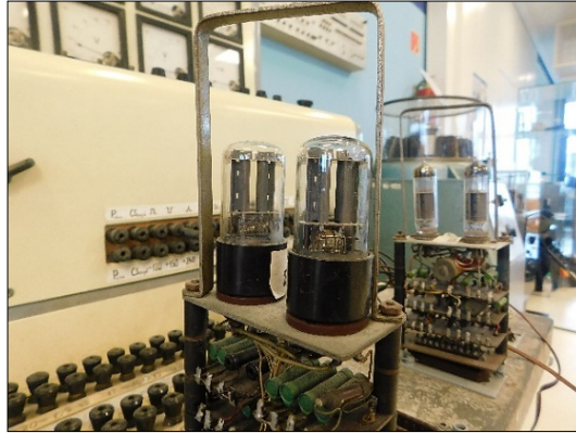
Fig. 12. Electron tubes from the first Hungarian von Neumann-inspired computer, M3. Photo: ajovomultja.hu
