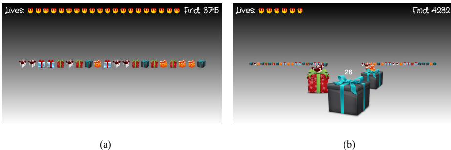
Fig. 4: Game for teaching search algorithms constructively. (a) An unsorted set of presents in which students must find the given number; a large number of lives is provided since a linear search will be required. (b) A sorted list; only a few lives are available, so students will need to use binary search to avoid looking at too many presents.
