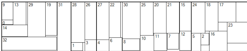
Fig. 6. Physical placement of AMI33, Unused area = 6.888%.
