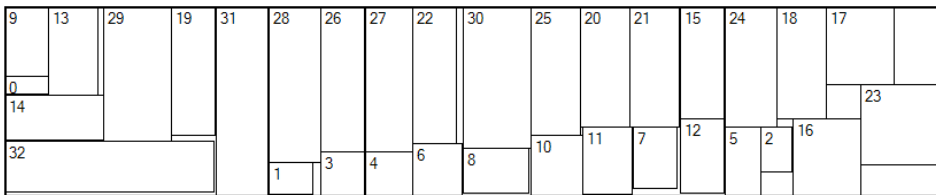
Fig. 6. Physical placement of AMI33, Unused area = 6.888%.
